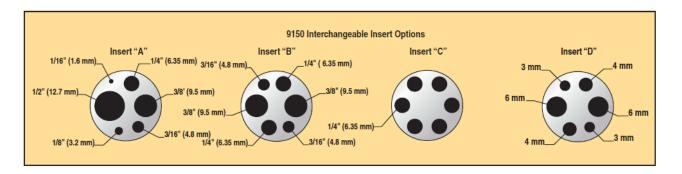
The 9150 Thermocouple Furnace uses Fluke Calibration's own microprocessor-based controller for great stability and set-point accuracy. It has a removable well insert for versatility. It has rapid cool-down and heat-up times. And it comes with an RS-232 port for connection to a PC.
