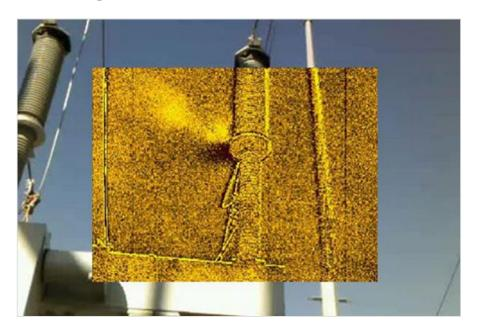
**FLK-Ti450 SF6 60Hz** Fluke Ti450 SF6 Gas Detector (60 Hz)
