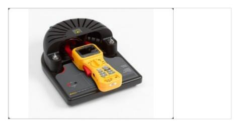
**52120A/COIL3KA**Coil, 25 Turn, 3000 Amp
