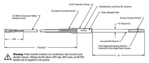
*Warning:* Probe handle surfaces are conductive. Use caution near electric circuits. Voltage levels above 30V rms, 42 V peak, or 60 V dc should not be applied to the probe.
