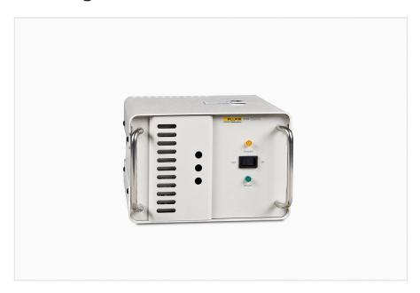
**9101**Zero-Point Dry-Well (includes one set of telescoping inserts to provide various smaller diameters)
